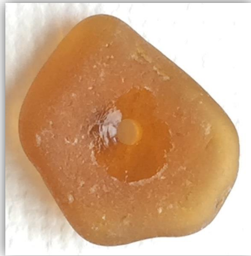
Left: Clean hole on initially drilled side of sea glass. Right: "Blow out" from drilling all the way through without counter drilling.
