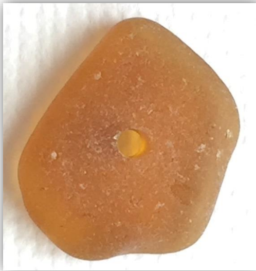
Left: Clean hole on initially drilled side of sea glass. Right: "Blow out" from drilling all the way through without counter drilling.
