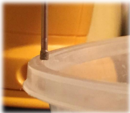
Drill bit at level so dish can slide on and off work area without tilting.
